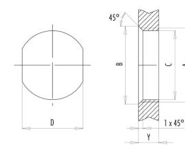
Installation direction: o-ring sits on chamfer.
